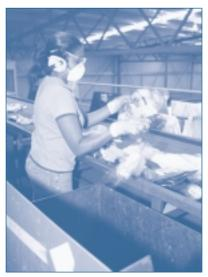
Materials sorted at the MRF for baling before being sent to industry for reprocessing.
